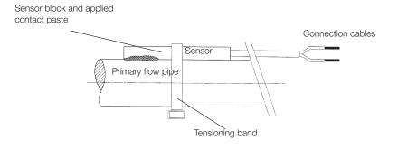
Do not permanently mount the sensor cable before you have tested and found the best position.
